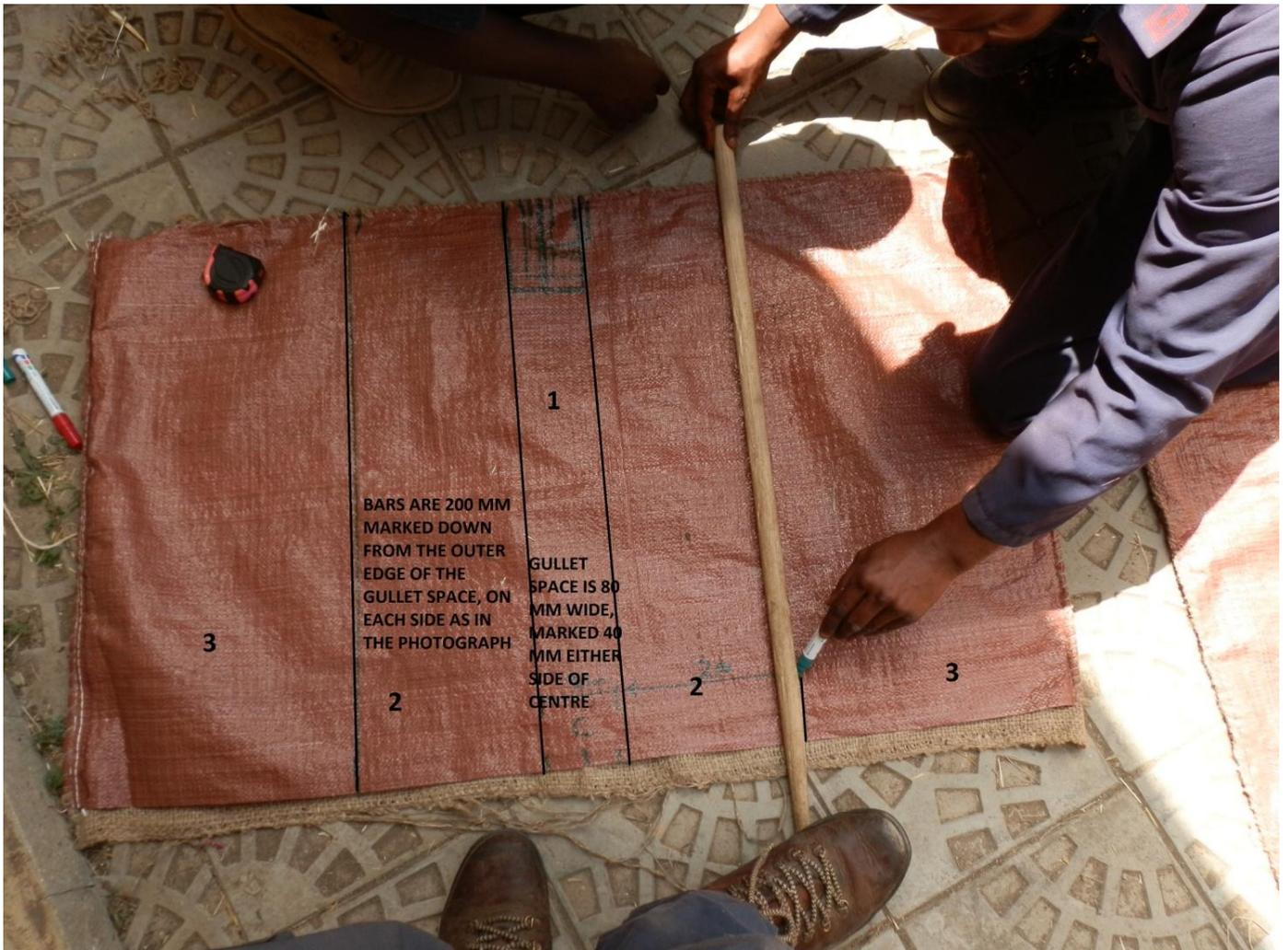
The Gullet 1/ is marked at 40 mm each side of the centre mark, so is 80 mm wide in total. The bars 2/ are measured at 200 mm from the gullet line down on each side. The panels 3/ are whatever is left, but should be equal, more or less.
